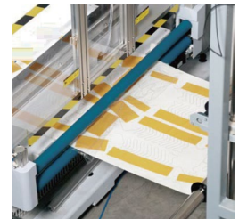
自动拉料装置 Automatic pulling device 自动拉料且能够压紧胶带 Automatically pulling the fabric, and pressing the tape firmly
