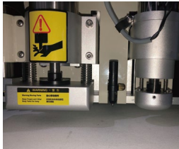
钨钢铣刀+刻字刀+钻孔刀 Multi-function cutting head
