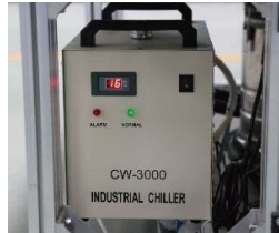
CNC水冷循环 CNC water cooling cycle
