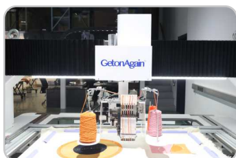
Lifting Tufting Head with Free Angle Rotation
