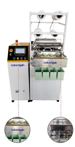
Temperature Control Box: For thermal treatment of bobbin thread after formation. 温控箱:
