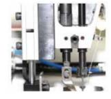
Use DLC coating needle bar and rotary hook shaft offer strong wear and abrasion resistance, lower friction with little or no oiling
