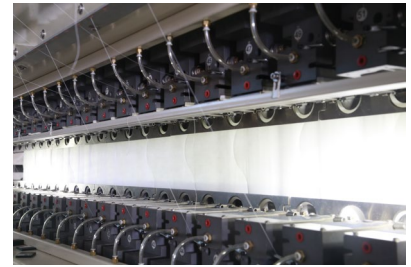
Double row machine: The unique adjustable hackle mechanism can make the pattern design more diverse. The row distance can be adjusted continuously from 75MM-210MM. The lower row head can be continuously moved horizontally, up to half the head spacing.
