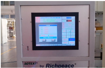
ARM+LINUX core, 15-inch touch screen, industrial-grade control system.
