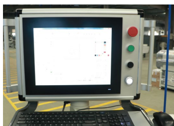
Control software is using MS Windows engineering interface, and compatible with CorelDraw, AutoCAD and other graphical output files format, can be used for various graphics marking, such as text and bar codes. Support a variety of common used graphic formats, such as AI, PLT, DXF, BMP, etc.
