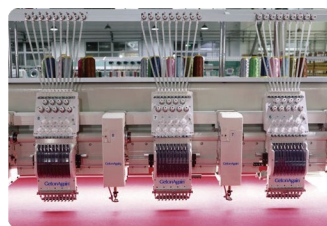
Latest thread clamping system and thread guiding tubes make it go more smoothly, lower thread breakage rate.
