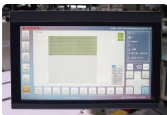
Model III control system, 15.6-inch LCD touch screen, refresh-rate with 50ms/time, real-time dynamic display.
