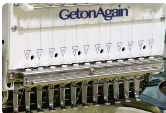
New upper thread holder: Reduce the thread breakage rate.
