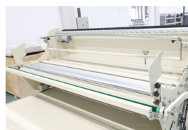
加大布斗850mm Enlarged Fabric Hopper 850mm
