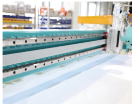
高精直线导轨, 保证机头、鞍架高速运行平稳 High precision linear guide rails ensure the sewing head and saddle running smoothly at a high speed
