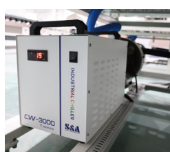
CNC水冷循环 CNC water cooling cycle
