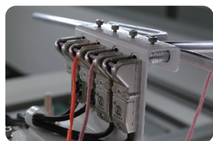
断线检测装置 Yarn Breakage Detection Device
