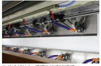
旋梭冷却结构,保证旋梭高速运行。 Rotary shuttle cooling structure ensures high-speed operation of rotary shuttle.
