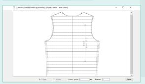
Software can output full-size pattern overlays as a mesh diagram in PLT file format.
