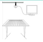
Spread the printed Black/White grid paper on the workbench and fix the camera on the top of paper.
