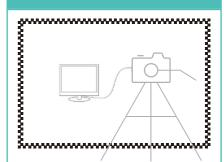
Fix the printed grid graph paper on the wall and fix the camera on front side.
