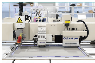
专用冲孔、绣作、缝制机头 Specialized Punching, Embroidery and Sewing Heads
