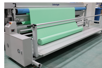
可选配全自动送料装置 Optional Fully Automatic Feeding Device: Available for increased efficiency.
